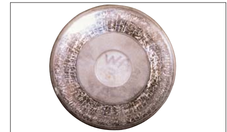
Photo 7-6-2 Part: Roller of a tapered roller thrust bearing Symptom: Thermal cracks occur at large end face of roller Cause: Heat generation due to sliding with the inner ring rib under poor lubrication
