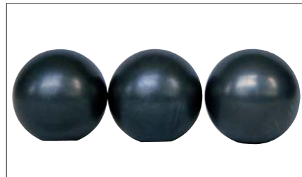
Photo 7-15-4 Part: Balls of a groove ball bearing Symptom: Electrical corrosion has a dark color that covers the entire ball surface
