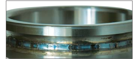
Photo 7-14-3 Part: Inner ring of an angular contact ball bearing Symptom: Raceway discoloration, melting occurs at ball pitch intervals Cause: Excessive preload
