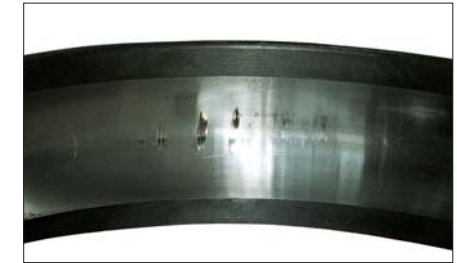
Photo 7-12-2 Part: Outer ring of Photo 7-12-1 Symptom: False brinelling occurs on the raceway Cause: Vibration from an external source while stationary
