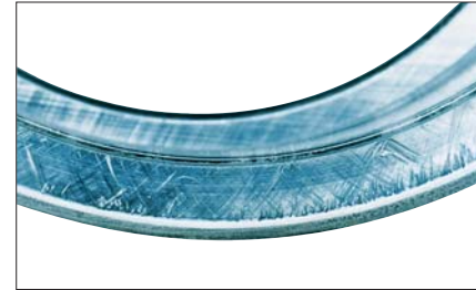
Photo 7-3-5 Part: Inner ring of a spherical thrust roller bearing Symptom: Scoring on the rib face of inner ring Cause: Debris, which is caught in surface, and excessive axial loading
