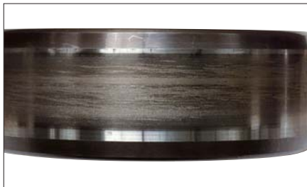
Photo 7-4-1 Part: Inner ring of a cylindrical roller bearing Symptom: Smearing occurs circumferentially on raceway surface Cause: Roller slipping due to excessive grease filling
