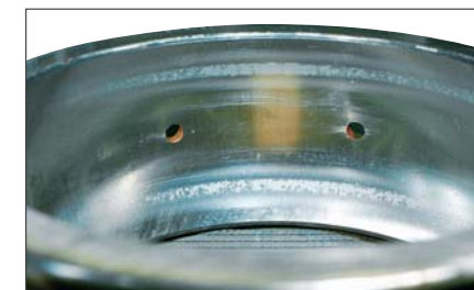
Photo 7-2-4 Part: Outer ring of a spherical roller bearing Symptom: Peeling occurs near the shoulder of the raceway over the entire circumference Cause: Poor lubrication
