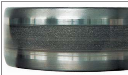
Photo 7-15-3 Part: Inner ring of a cylindrical roller bearing Symptom: Belt pattern of electrical corrosion accompanied by pits on the raceway surface
