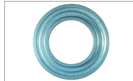
Photo 7-12-3 Part: Outer ring of a thrust ball bearing Symptom: False brinelling of raceway surface at ball pitch Cause: Repeated vibration with a small oscillating angle
