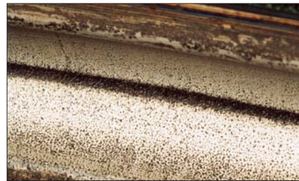
Photo 7-9-1 Part: Outer ring of a slewing bearing Symptom: Pitting occurs on the raceway surface Cause: Rust at bottoms of indentations
