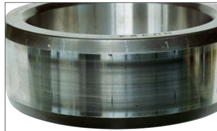
Photo 7-17-1 Part: Inner ring of a cylindrical roller bearing Symptom: Axial scratches on raceway surface Cause: Inclination of inner and outer rings during mounting
