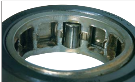
Photo 7-7-7 Part: Cage of a cylindrical roller bearing Symptom: Deformation and wear of a machined high-tension brass cage
