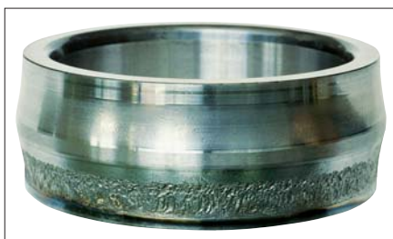
Photo 7-1-7 Part: Inner ring of a spherical roller bearing Symptom: Flaking of only one raceway over its entire circumference Cause: Excessive axial load
