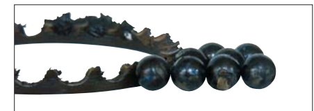
Photo 7-14-5 Part: Balls and cage of Photo 7-14-3 Symptom: Cage is damaged by melting, balls become discolored and melted Cause: Excessive preload
