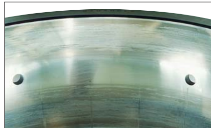
Photo 7-4-4 Part: Outer ring of Photo 7-4-3 Symptom: Smearing occurs circumferentially on raceway surface Cause: Poor lubrication
