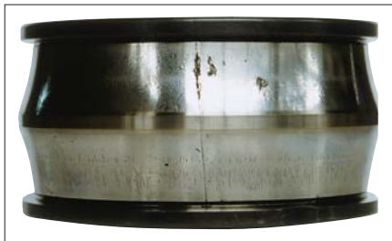
Photo 7-6-6 Part: Inner ring of a spherical roller bearing Symptom: Axial cracks occur on raceway surface Cause: Large fitting stress due to temperature difference between shaft and inner ring.
