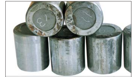
Photo 7-10-4 Part: Tapered rollers of Photo 7-10-3 Symptom: Stepped wear on the roller head and face Cause: Fretting progression due to excessive load while stationary
