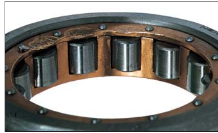
Photo 7-7-6 Part: Cage of a cylindrical roller bearing Symptom: Deformation of the side face of a machined high-tension brass cage Cause: Large shock during mounting
