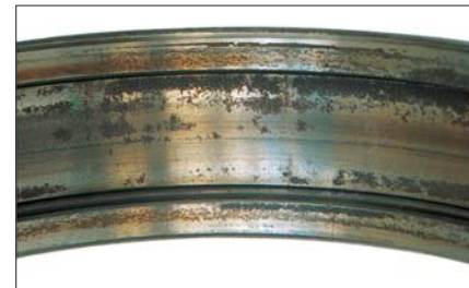
Photo 7-16-1 Part: Outer ring of a cylindrical roller bearing Symptom: Rust on the rib face and raceway surface Cause: Poor lubrication due to water entry
