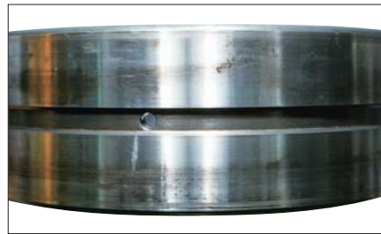
Photo 7-13-2 Part: Outer ring of a spherical roller bearing Symptom: Creep occurs over entire circumference of outside surface Cause: Loose fit between outer ring and housing
