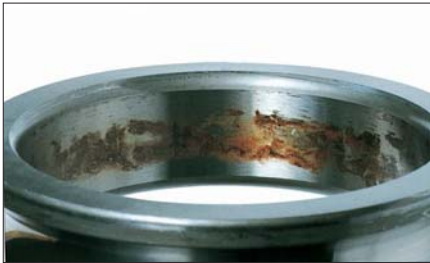
Photo 7-11-1 Part: Inner ring of a deep groove ball bearing Symptom: Fretting occurs on the bore surface Cause: Vibration
