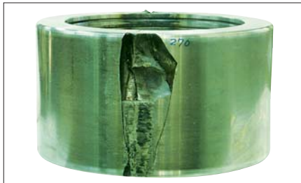
Photo 7-6-4 Part: Outer ring of a double-row cylindrical roller bearing used for outer ring rolling (Outer ring rotation) Symptom: Cracks occur on outside surface Cause: Flat wear and heat generation due to non-rotation of the outer ring
