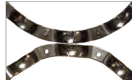
Photo 7-7-1 Part: Cage of a deep groove ball bearing Symptom: Fracture of pressed-steel cage-pocket
