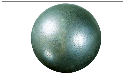
Photo 7-9-2 Part: Ball of Photo 7-9-1 Symptom: Pitting occurs on the rolling element surface
