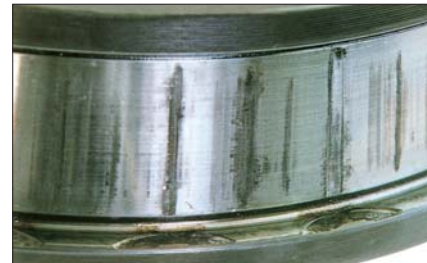
Photo 7-10-3 Part: Inner ring of a double-row tapered roller bearing Symptom: Fretting wear of raceway and stepped wear on the rib face Cause: Fretting progression due to excessive load while stationary
